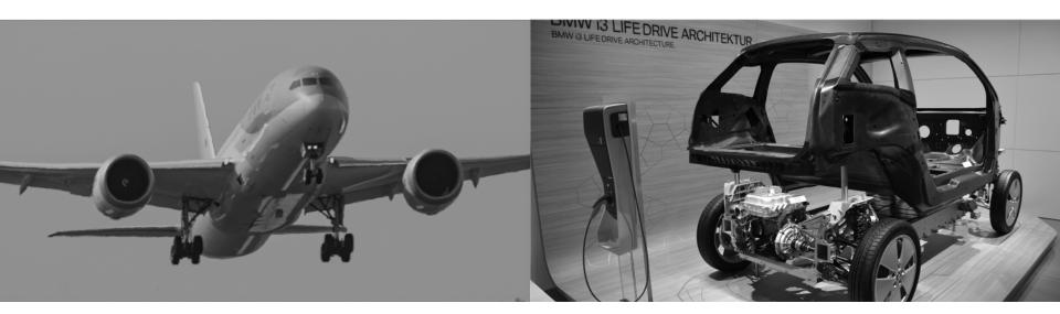
The Boeing 787 Dreamliner airframe is nearly 50% carbon fiber reinforced plastic and other advanced composites<sup>1</sup>
