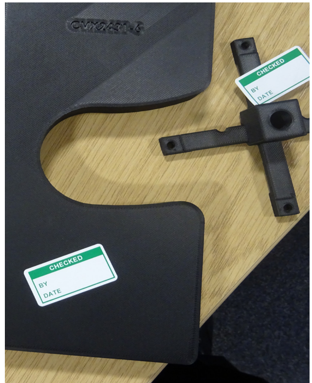
The team has replaced several parts with 3D printed parts using Markforged's Onyx material
